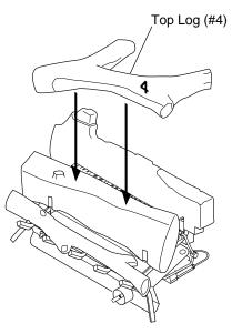
Figure 20 - Installing Top Log
